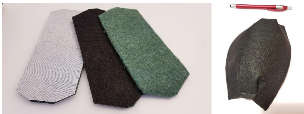
Biocidal insert coated with standard PP material filtering particles
